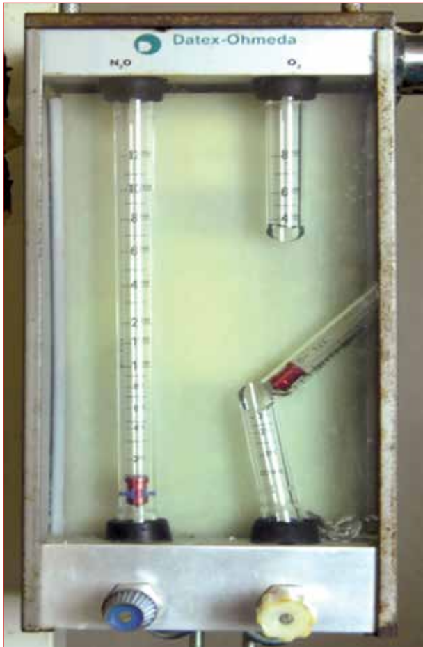
Figure 1: The broken oxygen flowmeter
